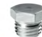
Plugs for subsequent closing of boreholes are usually made of steel, zinc-plated and passivated, with tapered thread. Available in many different types.
