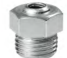
Pressure relief for releasing excessive pressure in gearboxes or bearing housings are usually made of steel, zinc-plated and passivated, with tapered thread. Available in many different types.
