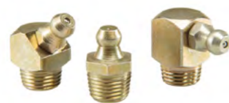
Hydraulic type grease nipples with self-tapping thread, Form A, B, C (180°/45°/90°). Specially surface hardened to prevent abrasion.
