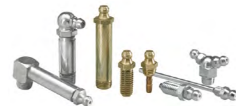
Hydraulic type grease nipples special designs in any kind of different dimensions, thread sizes and forms, manufactured in all feasible materials. Amongst others available with pin valve, check valve, extension or double-head.
